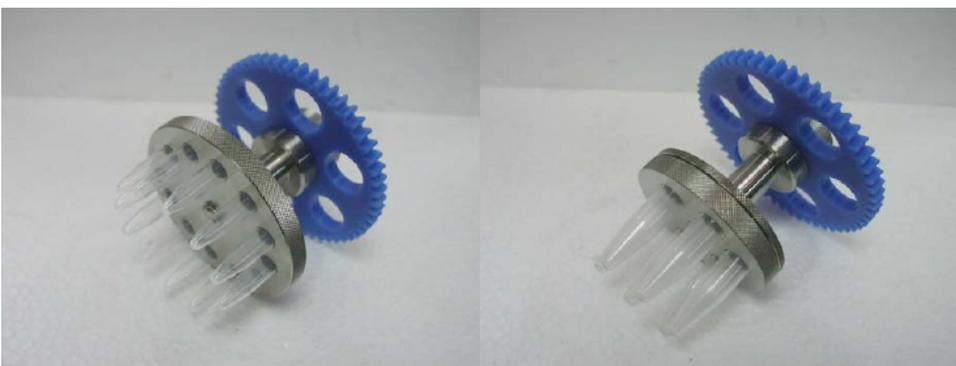
**Figure 1: Tube holders for use in the Bioruptor**
